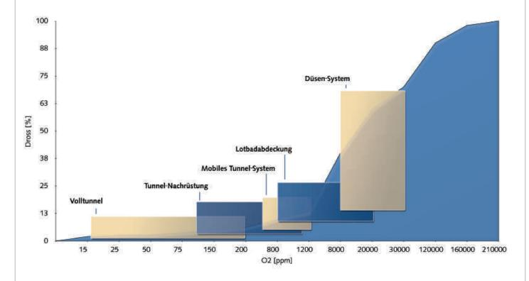
Wave soldering systems can be inerted in a variety of ways. A distinction is generally made between three of these.
