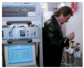
Connecting calibration gases at the measurement station
