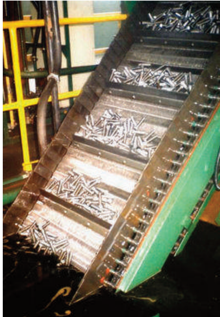
Fig. 7: Hardened screws leave the oil bath.
