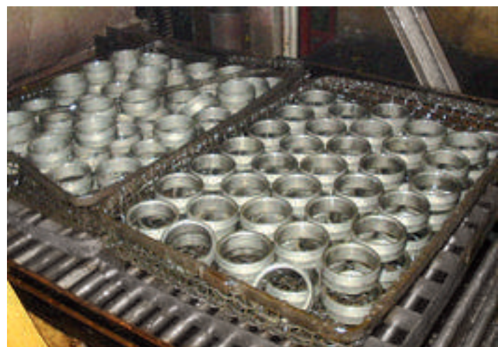
Fig. 5: Annealed bearing rings of 100 Cr6 steel
