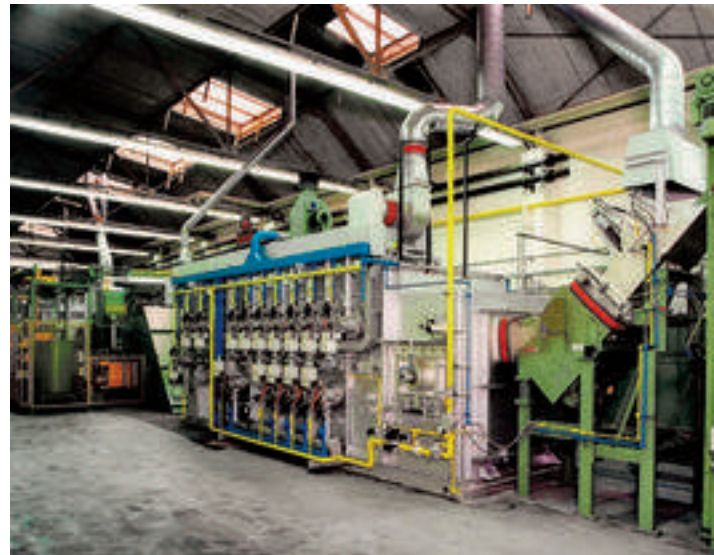
Fig. 4: Continuously conveyor furnace from Aichelin
