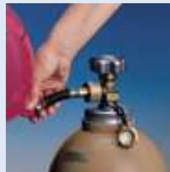
3. Push balloons on to the filling nozzle, bend the valve down slightly and carefully let the gas flow into the balloon until it has reached the desired size (Caution, high pressure).
