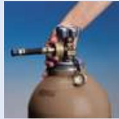
2. Screw inflation valve on to cylinder valve by hand (do not use a tool!) Open cylinder valve (slowly). Check that the connection is tight.
