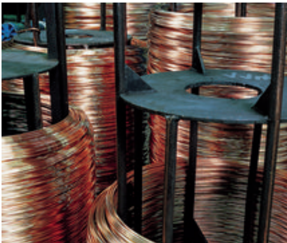
Soft annealed copper wire in a bell-type furnace
